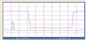
Minimum width of discriminator input signal: 2 ns pulses with 5 mV overdrive are captured with 99.9% efficiency. Actual behavior is better as for this test we use the output of the shaper (with 1 mV r.m.s. noise as reference for comparator). Delay due to pulser trigger.
