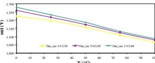
Plot of the common mode differential output (120 Ohm load) versus temperature for three power supply choices.
