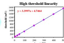
Time walk about 3.5 ns @ threshold 1.5 fC (input charge range: 1 fC - 1 pC).
