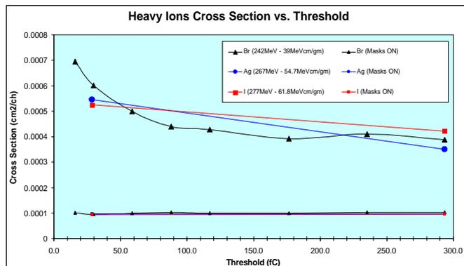
Figure 6: Heavy ions cross-section versus threshold.
