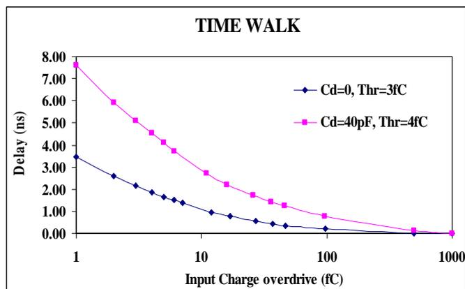
Figure 3: Time walk of the bare chip with 2 input configurations.
