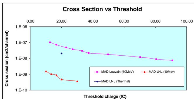
Figure 5: Fast and slow neutrons cross-section versus threshold.
